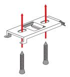
Fix the brackets to the ceiling or the underside of the lintel using two screws. Place the brackets evenly along the width of the track to offer support.
