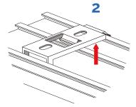
Push the back of the track upwards until you hear a click as the bracket locks onto the rear two ribs of the track.
