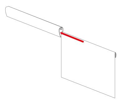
Push the end cap onto the runner to lock the panel in place and secure the end cap with the small screw.
