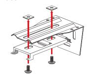
For face fixing, assemble the unit by attatching the bracket to the 'L' shaped plate.
