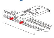
Rest the track on the front prongs of the bracket, they locate on the first rib along the top of the track.
