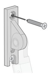
If you need to adjust the position of the spring arms, loosen the screw in the bottom of the spring-arm bracket slightly and adjust up and down as necessary.
