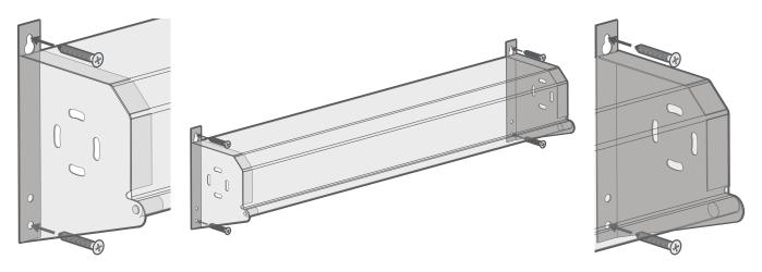
Use the top and bottom screw holes on the back of the cassette to face-fix the cassette to the wall.
