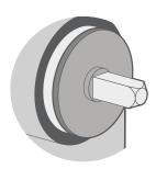
Take the roller and slot the square peg on one end into the square slot on the inside face of the crank mechanism.
