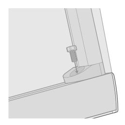
Curl the bottom bar back and slot the channel on the bottom of the bar onto the pegs on the bottom of each spring arm. Secure the arms to the bottom bar with the fittings provided.
