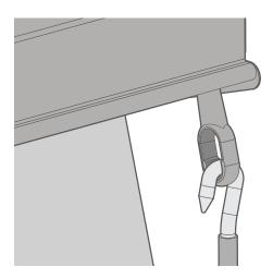
Hook the crank handle onto the crank mechanism and use it to fully lower the blind.
