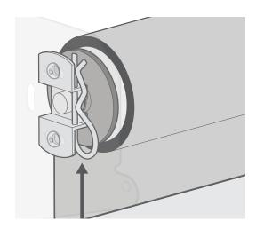
Secure the pin by inserting the R-clip into the roller plate.
