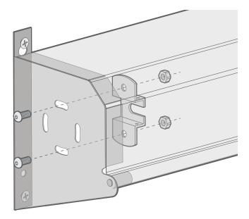
Use two short bolts and two nuts to attach the roller plate to the inside of the cassette. The notch in the plate should be facing toward you.
