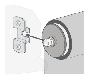
Slot the roller pin into the notch on the roller plate.
