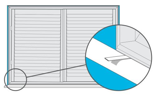
The best method for adjusting the level of the panels is actually to adjust the frame. If one panel sits higher than the other, go to the side which is sitting lowest and loosen the frame screws on that side, and along the bottom. Then insert one of the frame shims from your fixing kit to raise that side slightly. This should level out the panels.
