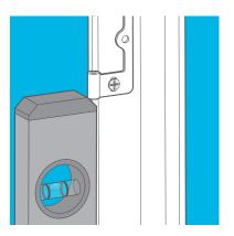
Make sure you also use the spirit level on the front of the frame, on all sides, to ensure there's no 'twist' to the frame.
