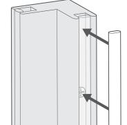
For Inside Recess frames, reinsert the decorative strips you removed in step 2.
