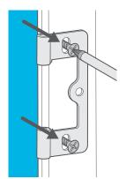
Start by loosening the frame hinges, as this will make aligning the two parts of the hinge easier (one part is fixed to the frame, the other part is fixed to the panel). This will also allow you enough room to slot the hinge pins into place.
