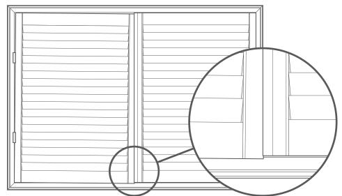
Because no recess is perfectly square, you'll likely find that some adjustments are required to align the panels (i.e. if one panel sits slightly higher than the other), although thorough checks with your spirit level throughout the installation process should help to minimise the amount of fine tuning required.
