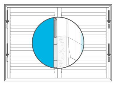
Now slot the hinge pins into place. Starting with the top hinge on each panel, align the panel part of the hinge with the frame part of the hinge, then insert the pin through the centre. If your shutter has folding panels, join these together the same way.
