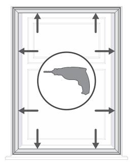
Making sure that the frame stays still and level, push the drill through each of the fixing holes you made in the frame and drill a small pilot hole in the surface you're fixing the shutter to (the inside of the recess). Drill through the plaster as far as the timber beneath. You should now be left with shallow pilot holes all around the recess - two for each side, the top and the sill.
