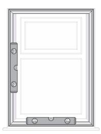
Place the assembled frame in the recess and use a spirit level to make sure that it is sitting perfectly straight on all sides.
