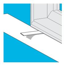
If you need to adjust the level of the frame then you can use the frame shims from your fitting kit. Fully insert the shim so that it is hidden by the
