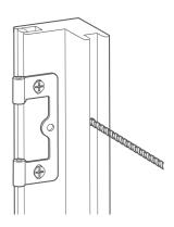
For 'Inside Recess' fitting, remove the decorative strip covering the channel toward the back of the frame and drill your holes inside this channel.
